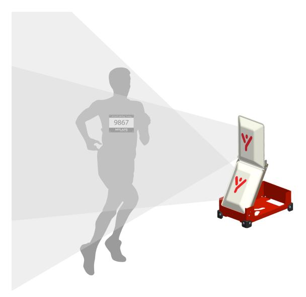
Because of the unique dual antenna design of the MYLAPS BibTag Side Antenna it has the highest read rates. The upward angle and positioning close to the ground avoids core body interference and the dual angles further enhances the performance.
