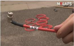
BNC connectors are on both ends of the cable. One end is right angle shaped and one end is straight. The right angle end connects to the decoder and the straight end connects to the mat.
