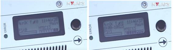
If a mat is not detecting the Tag, check the antenna cables and either replace them or the mat if necessary and repeat the test.
